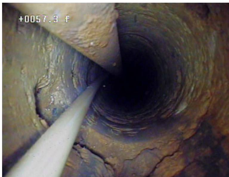
Figure 10: Video log image of the pipes under water which also shows staining on the borehole walls.
