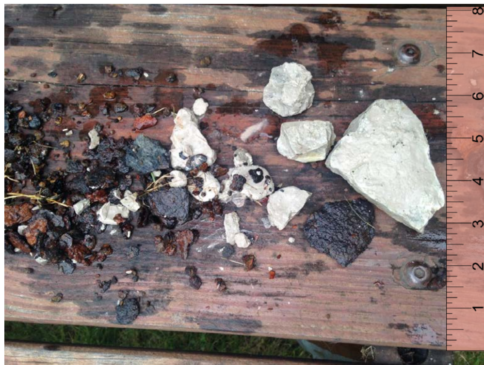
Figure 23: Typical sediment removed from the well during the air lift process. The largest piece of dolomite is just over 3 inches across.
