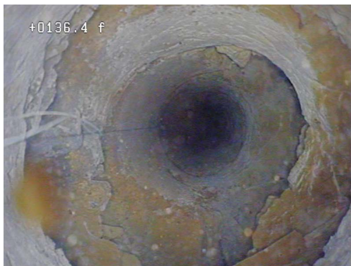
Figure 26: Video image showing some of the many open fractures in this borehole.
