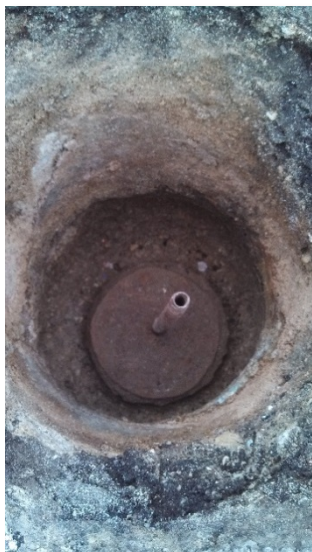
Figure 31: Steel plate with 1/4-inch access port.
