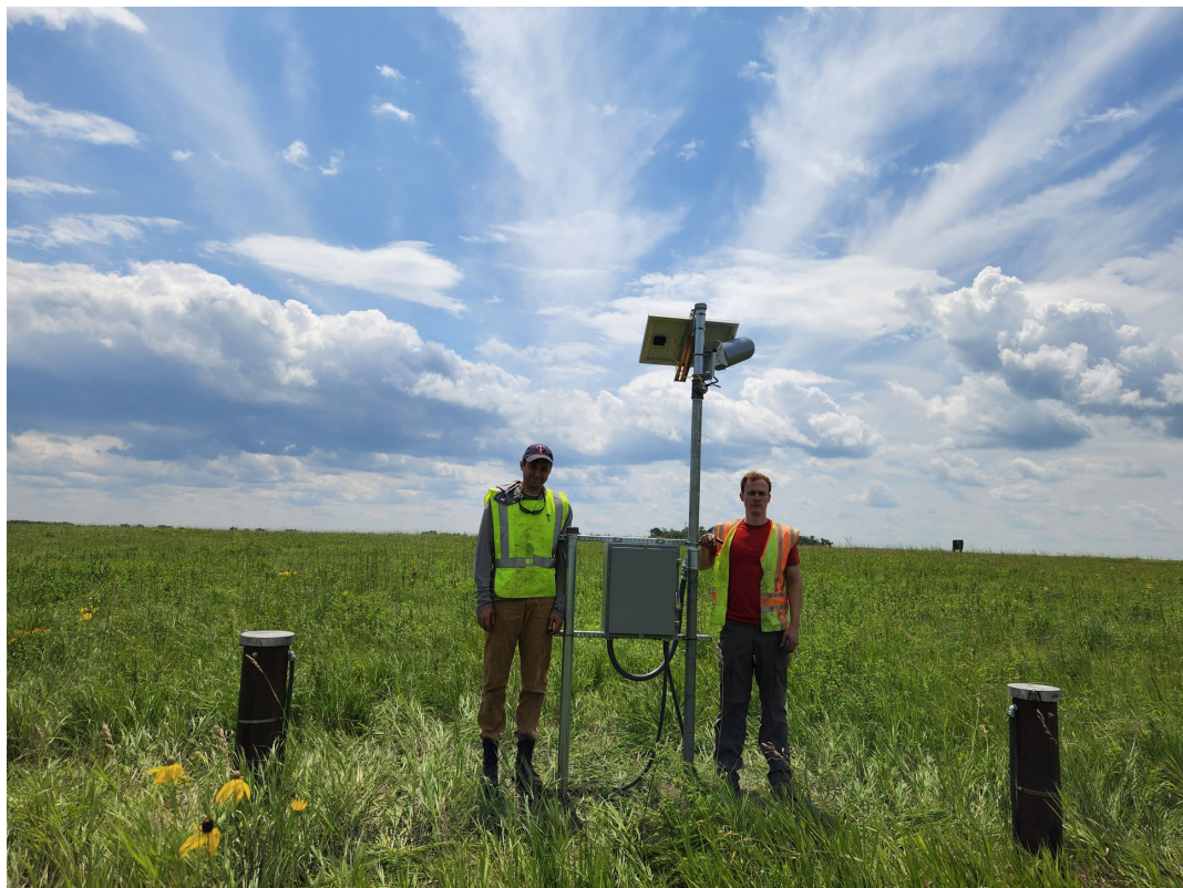
Figure 1: A site photograph of a newly installed GOES satellite telemetry setup at an observation well nest in Stearns Co, MN.
